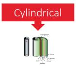
A spirally wound design (jelly-roll). Designated by size, e.g. 26650 cylindrical battery (Diameter: 26mm, length: 65.2 mm; code for cylindrical shape: 0)
