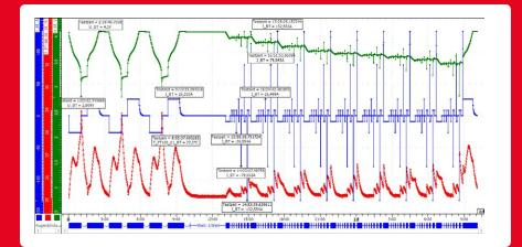
In order to select a particular cell type for a specific application, it is first necessary to measure the nominal capacity of a cell and thus compare it with the manufacturer's specifications. In a second step, the temperature-dependent cell resistance is determined in a wide range from -20 to 50°C.
