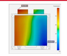
The temperature dispersion within the cell is simulated under current load. The knowledge gained is used to develop efficient cooling and operating strategies to avoid cell-damaging hot spots. The developers are now able to select exactly that cell that is best suited for the respective application.
